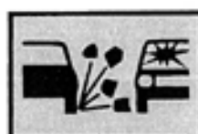
Loose stones on roadway. Danger of windscreen damage - slow down, exercise caution.
