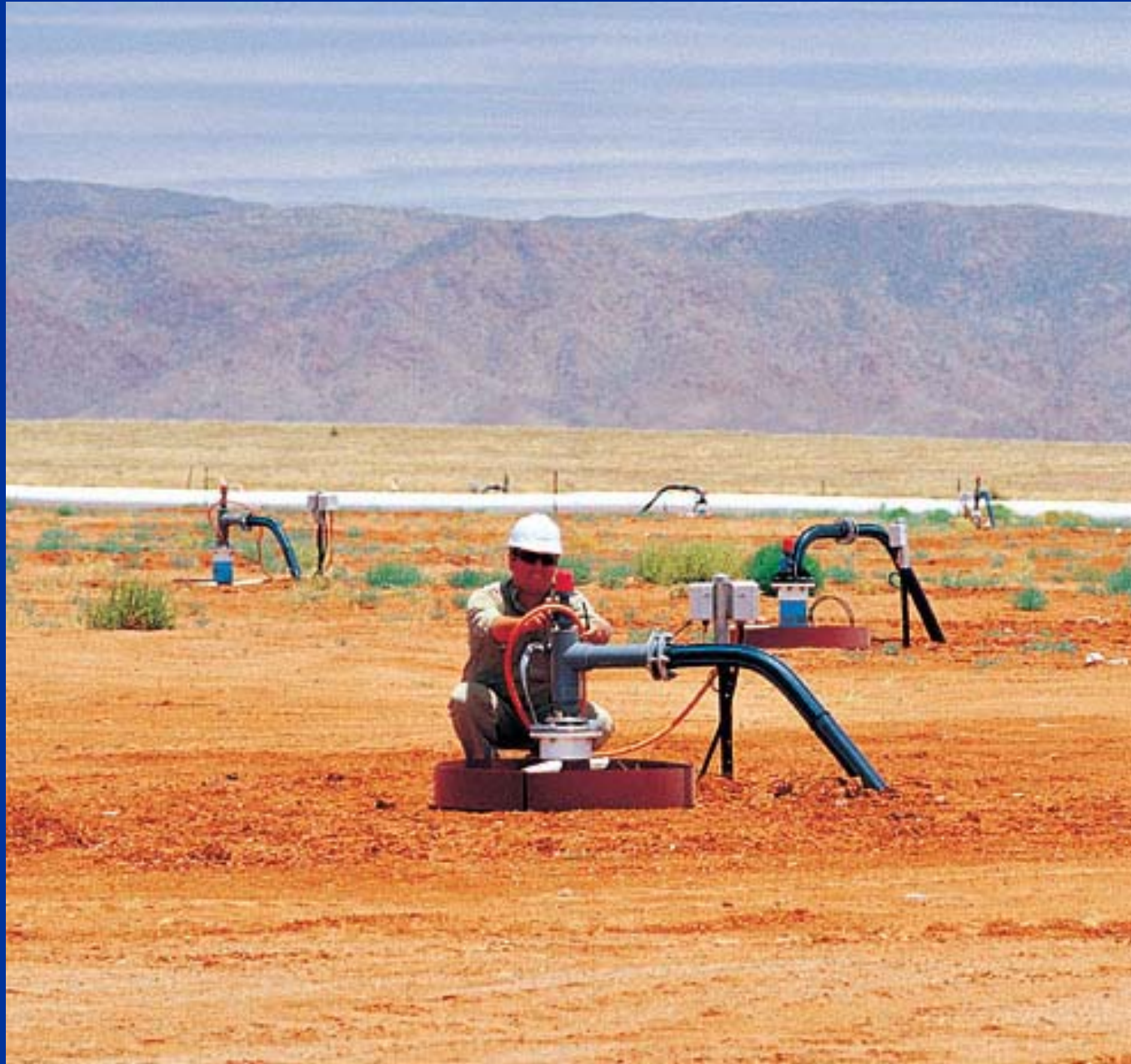
Beverley Uranium Mine in-situ leach recovery
